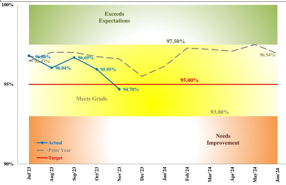
**Rail Mean Distance Between Failures** measured as the average rail car miles between NTD reportable mechanical failures, i.e., those precluding a rail car from completing its revenue trip or starting its next scheduled revenue trip.
