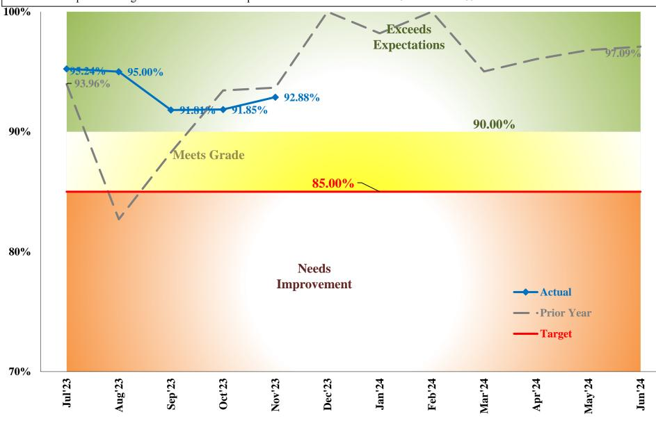
Streetcar Mean Distance Between Failures measured as the average actual vehicle miles (revenue + deadhead miles) between major mechanical failures reportable to NTD, except for those that occur at the end of the line.
